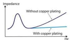
Furthermore the pole piece is copper plated in the magnet gap in order to reduce eddy currents. The purpose of this is to obtain linear impedance throughout the full frequency range and thus a linear treble reproduction.
